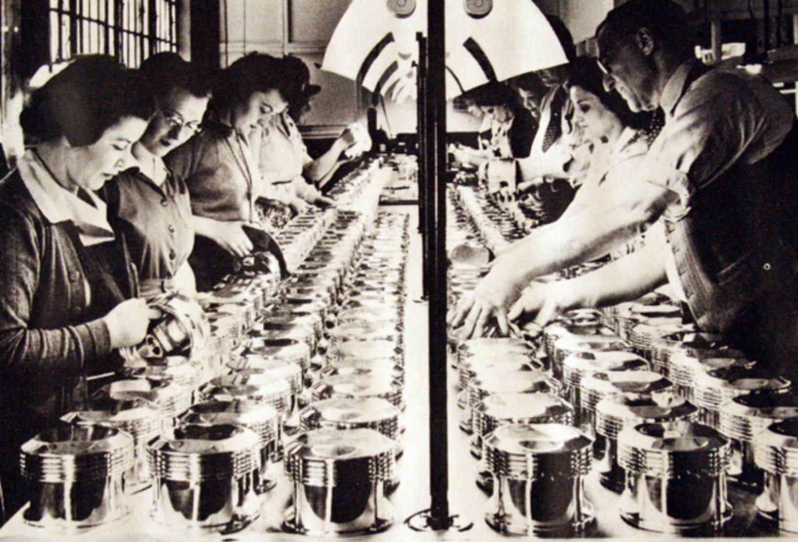
Hudson produced over 1 million Wright Cyclone aircraft engine pistons during WWII
