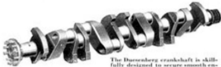
The Duesenberg crankshaft is skillfully designed to secure smooth engine operation and long bearing life.
