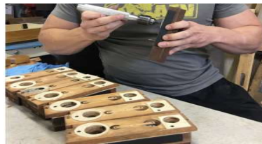
Reassembling the finished Casavant Primary blocks with all new gaskets, valves, and pneumatic leather.
