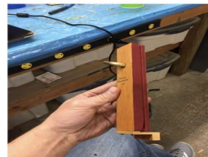
The same stop switch releathered and ready for installation.
