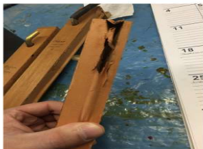
A 1960's stop control switch (not from Zion's organ) showing the tears that have developed, rendering the entire stop dead.
