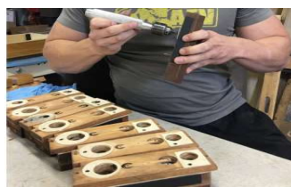
Reassembling the finished Casavant Primary blocks with all new gaskets, valves, and pneumatic leather.
