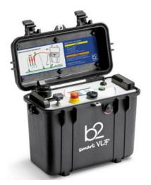
The HVA28TD are truly compact and portable VLF test sets for testing of medium voltage cables.
