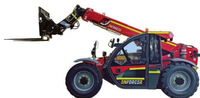
Model: THDBXH30-17K2XS Lifting Capacity: 3000kg
