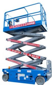
GS1932m Electric Narrow Scissor Lift: 5.55 m
