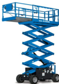
GS4069 BE Bi-energy Rough T Scissor Lift: 12.12 m
