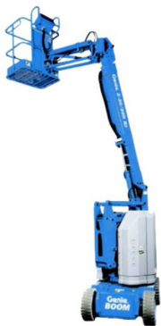
Z-30/20N Electric Articulating Boom Lift: 9.14 m
