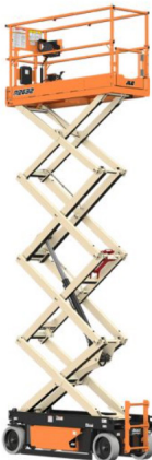
R2632 Electric Narrow Scissor Lift: 7.8 m
