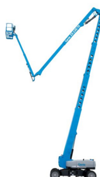
ZX135/70 Diesel Articulating Boom Lift: 41.15 m
