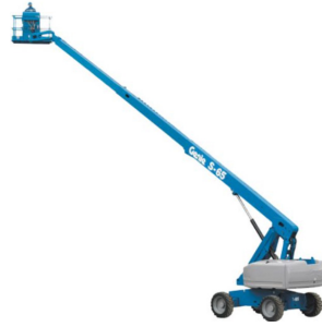
S65 Diesel Telescopic Boom Lift: 19.8 m
