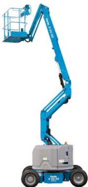
Z-34/22N Electric Articulating Boom Lift: 10.52 m
