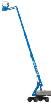
S65 XC Diesel Telescopic Boom Lift: 19.81 m
