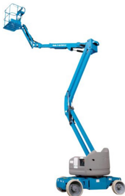
Z-40/23 N RJ Electric Articulating Boom Lift: 12.32 m
