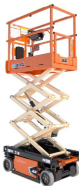
R3246 Electric Scissor Lift: 9.8 m
