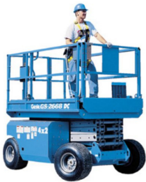
GS3268 DC Electric Wide Deck Scissor Lift: 9.75 m
