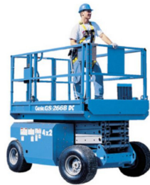
GS2668 DC Electric Wide Deck Scissor Lift: 7.92 m
