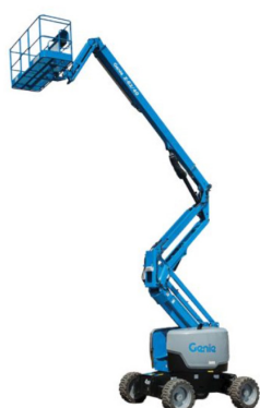
Z-62/40 Diesel Articulating Boom Lift: 18.87 m
