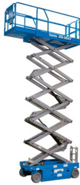
GS4047 Electric Scissor Lift: 11.7 m
