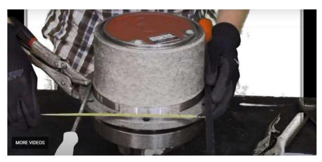
How to measure the distance between center hole on either side on bottom flange.
