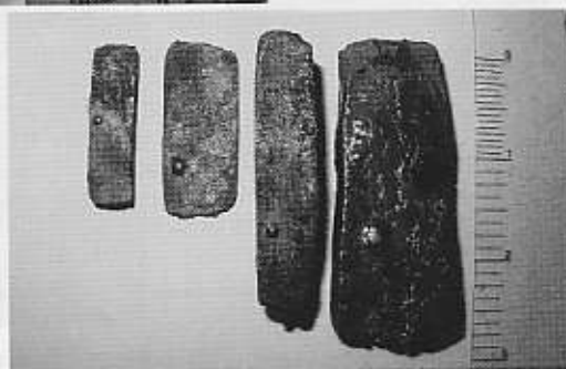
Copper ingots showing the mysterious bubble that sometimes forms on copper ingots.
