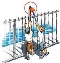
11. When the release mechanism of the self-latching device is located less than 54" from the bottom of the gate, the release mechanism shall be located on the pool side of the gate at least 3 inches below the top of the gate. ICC 3109.4.1.7
