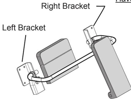
Depress brake pedal in parking brake position. Assemble Cart Lock as shown and position with locking bar over brake pedal and under gas pedal. Note\*\* On Club cars, brake must be in bottom most position.
