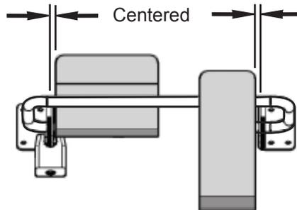
Center unit left-to-right between pedals. **Keep locking bar level.**
