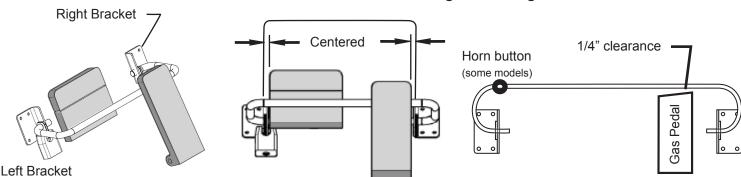
Depress brake pedal in parking brake position. Assemble Cart Lock as shown and position with locking bar over brake pedal and under gas pedal.
