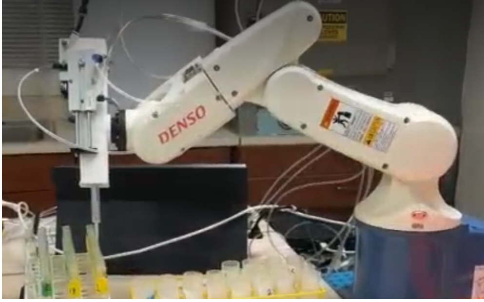
Fig. 7 Example of a robotic-assisted laboratory platform for automated liquid handling and sample manipulation. Robotic systems may support future automated microscopic sample preparation and image acquisition workflows for Arthrospira platensis monitoring applications, reducing manual handling variability and improving operational consistency.
