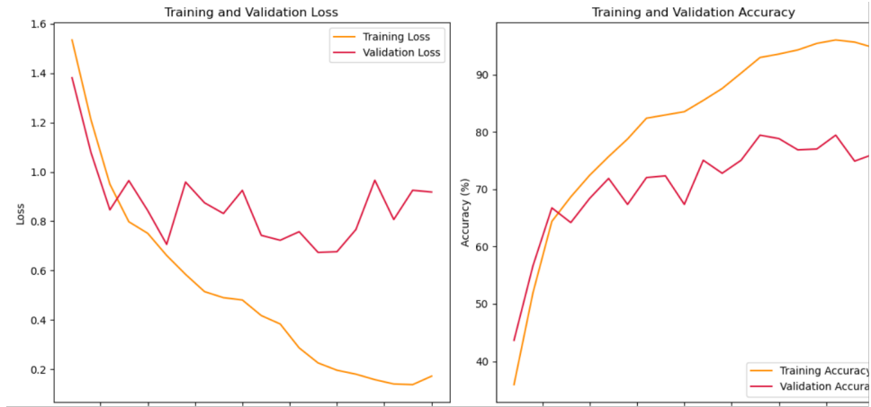
Fig. 8 Training and validation loss and accuracy curves obtained during CNN training using the ResNet50 transfer learning architecture. The loss curves illustrate the optimization behavior of the model, while the accuracy curves demonstrate the classification performance evolution across training epochs. The observed fluctuations in validation accuracy suggest the presence of dataset variability and limited generalization caused by the relatively small microscopic image dataset.
