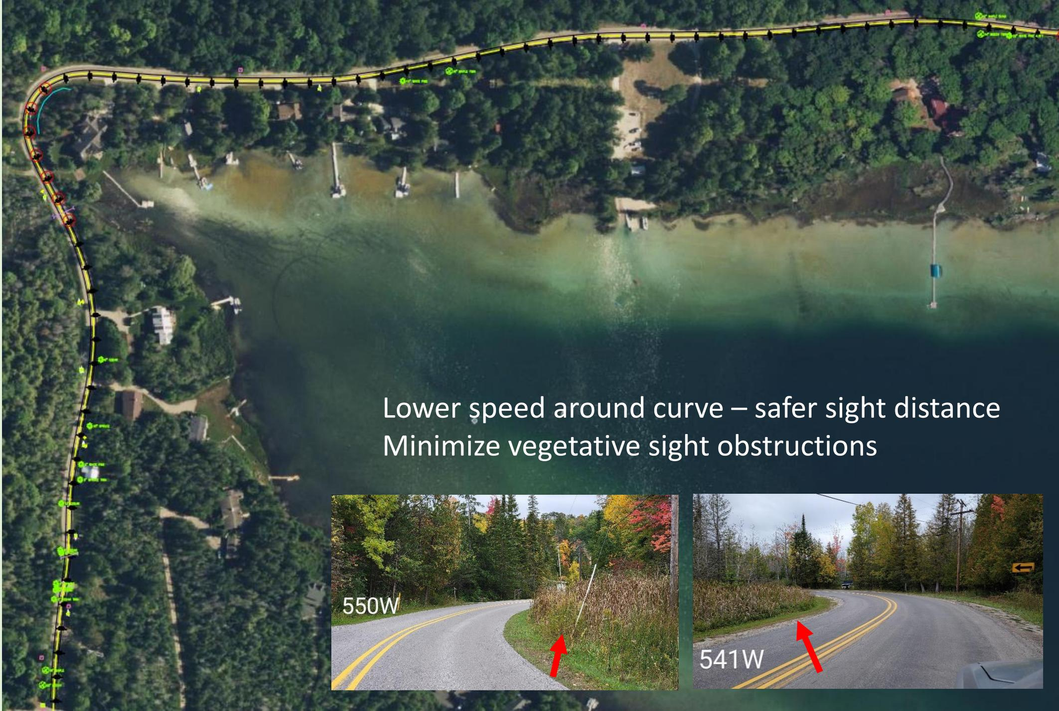
Lower speed around curve – safer sight distance
