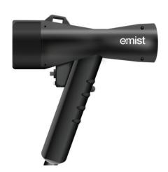
The EM360 is the most powerful, efficient and cost-effective disinfectant application system in the world. This patented system places a positive electrostatic charge to the disinfectant as it leaves the spray nozzle, causing each droplet to become powerfully attracted to its opposite charge on such high-touch areas as desks, table tops, chairs, door handles, cabinet handles, light switches and more. Using the EM360, you can help stop the unnecessary spread of infections.
