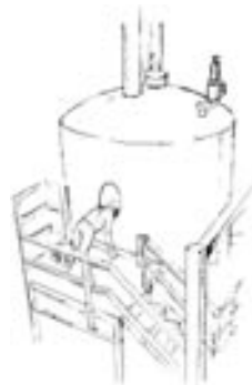
This process vessel at a pulp mill is a confined space. One worker died inside the vessel from lack of oxygen, and another died with his head in the opening.
