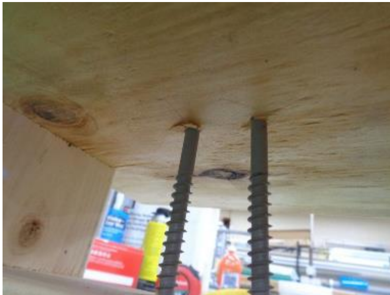
Photo No. 14 ASTM D1970 Specimen at Test End
