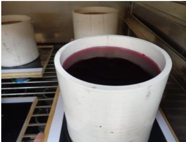
Photo No. 11 ASTM D1970 Specimens in Chamber
