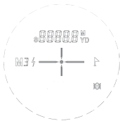
Figure 3 Ranging lock + vibration
