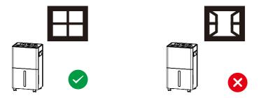
3. By placing the dehumidifier in the center of the room, you allow the air to circulate around the unit. Ideally, you should aim for about 18 inches of space around all sides of the unit.
