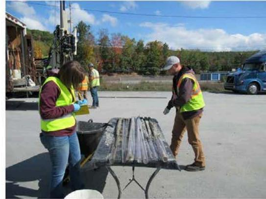
16.) View North - Groundwater Purge and Sampling of One (1") Inch *GeoProbe* Soil Boring Obtained for STARS 8260 / 8270 Laboratory Analysis.
