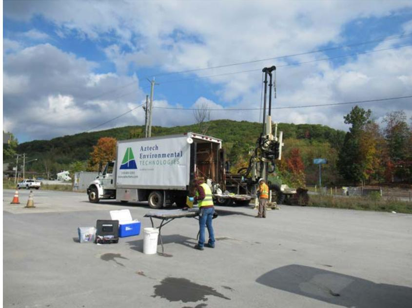
10.) View Northeast – Soil Coring to Approximately 20 Feet – Photo Depicts Soil Sample Boring and Groundwater Sampling Southwest and Downgradient of the Diesel Tank Area.
