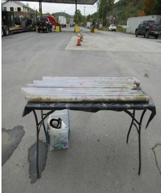
**12.) Soil Coring Sleeved Sliced Open - Inventoried & Documented for Assessment by PID, Visual and Olfactory Methods.**
