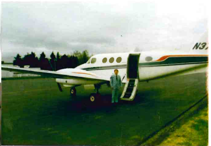
Inland Owned and Operated Aircraft Beechcraft King Air F-90 Turbo Prop All Weather Full Instrument 8 Passenger
