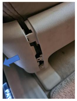
b. Squeeze the two clips on the inside of the center trim to release the trim from the seat metal frame
