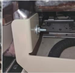
7. Make sure that the bracket is resting properly on the two front sides of the seat frame
