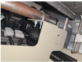
5. Partially remove the seat side trim by releasing the 4 clips in red circles
