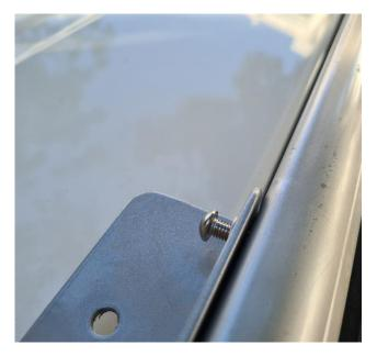
7. Tighten the two bolts using the hex key.
