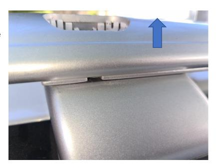
6. Screw in the two hex bolts included (One replaces the bolt you removed and one for the side of the rail) using the Hex key provided, do not forget the small washers, do not reuse the factory bolt again
