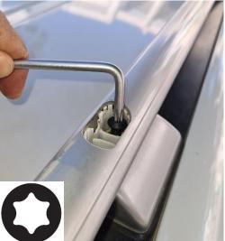
5. Now slightly lift the rail hand to create clearance between the rail and the middle fixing base, slide the Rahala flag bracket between the roof rail and the base, make sure the guide pin in the base passes through the slot in the bracket.
