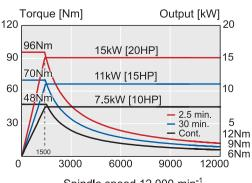
Spindle speed 12,000 min<sup>-1</sup>
