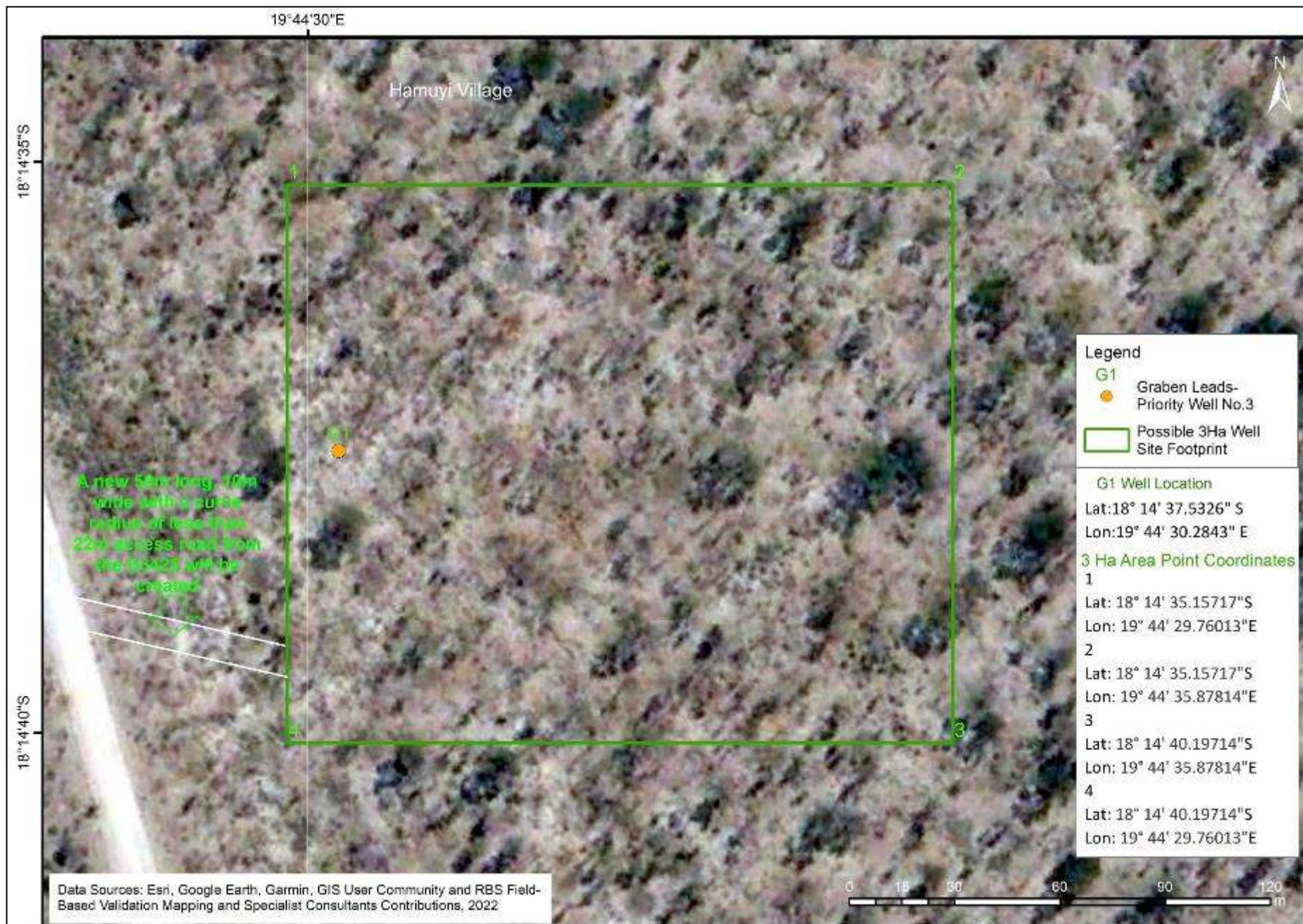
Figure 1.31 Detailed outline of the 3Ha area of the priority 3 for the Graben Play covering the Karoo Rift Fill and Intra-Rift Fault Blocks Leads proposed exploration and appraisal well location No. G1 located at Hamweyi Village along the eastern side of the D3425 road linking Rundu to Ncaute. A new 50m long, 10m wide with a curve radius of less than 22m access road from the D3425 will be created.
