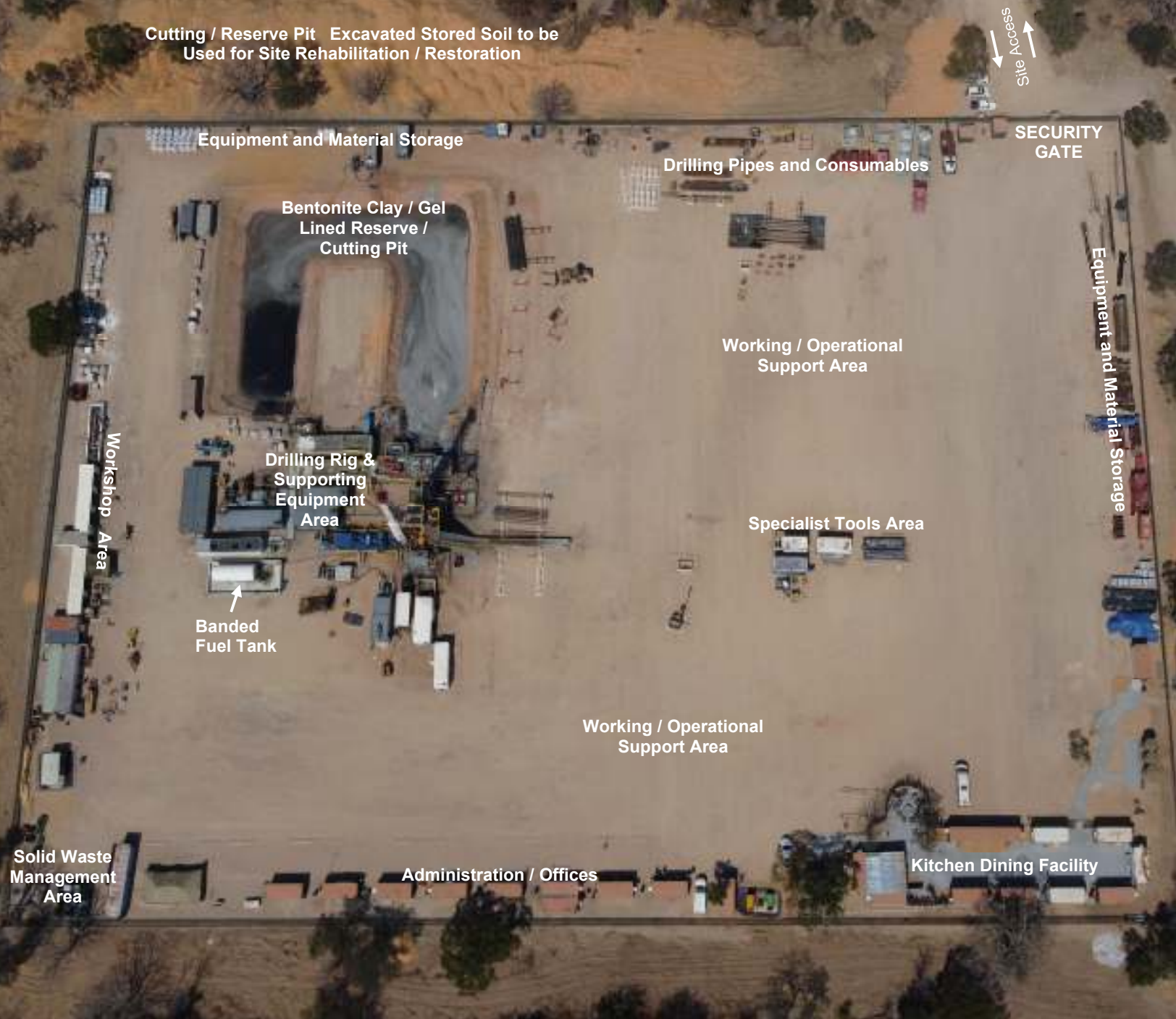
Plate 3.3: Example of an oil and gas well site layout showing a drone view of the 8-2 Makandina well site in Kavango East Region.
