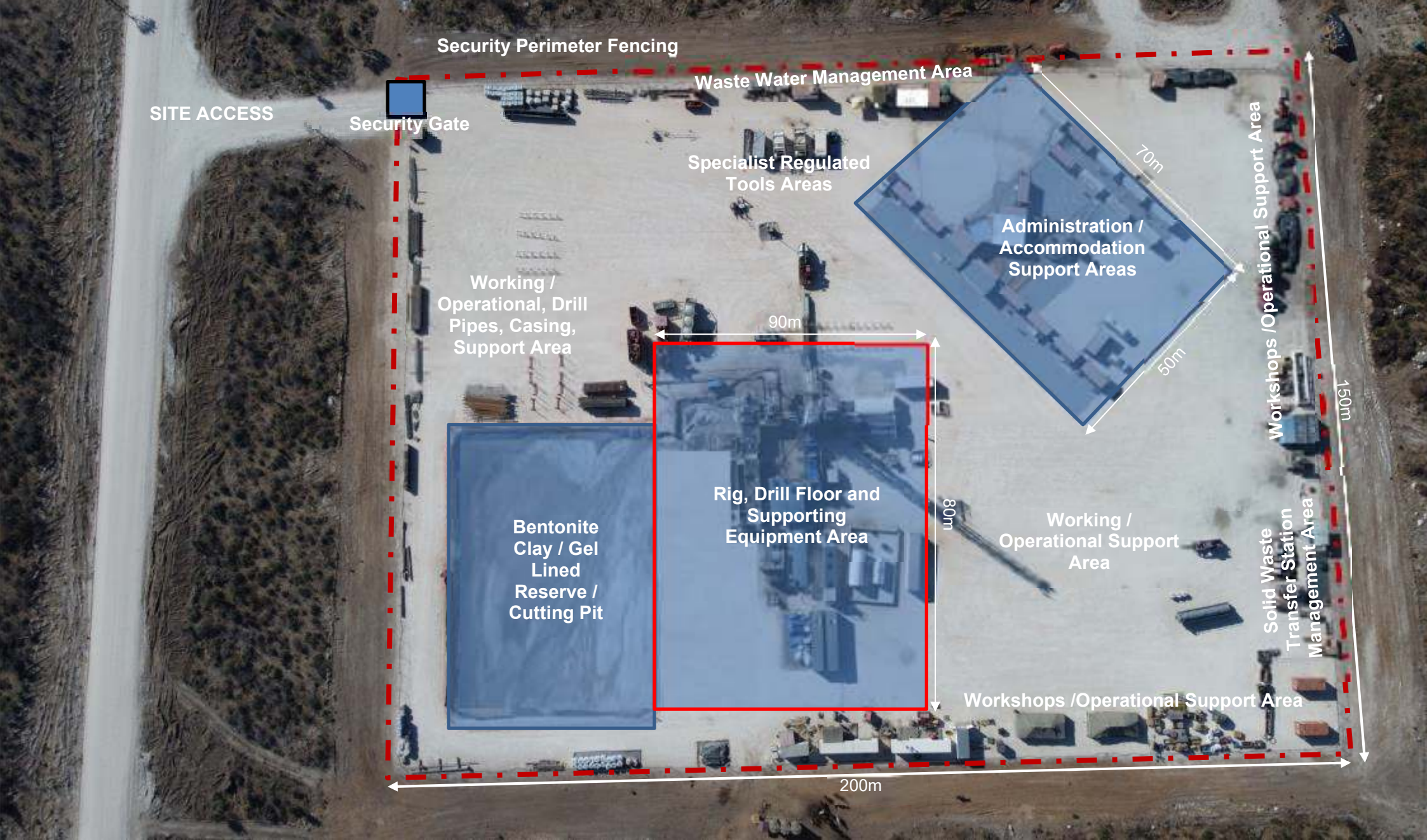
Figure 3.4: Layout example of a typical 3Ha footprint created by an onshore drilling well site coverage superimposed on an actual drilling location and as adopted for the drilling of multiple exploration and appraisal wells within the AOI in PEL No. 73 (Drawn not to scale).
