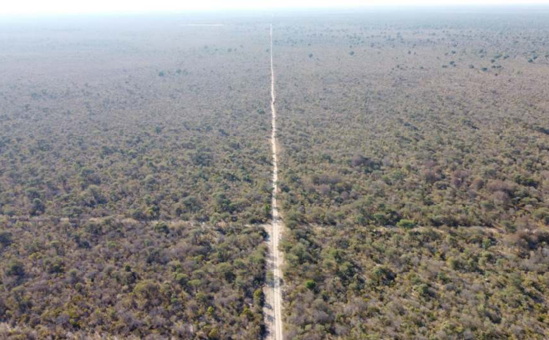
Plate 1.1: Drone image showing the example of the types of existing accesses that will be upgraded to a 10 m wide with a curve radius of less than 22m to be linked to the new access road to be created for the proposed well locations.
