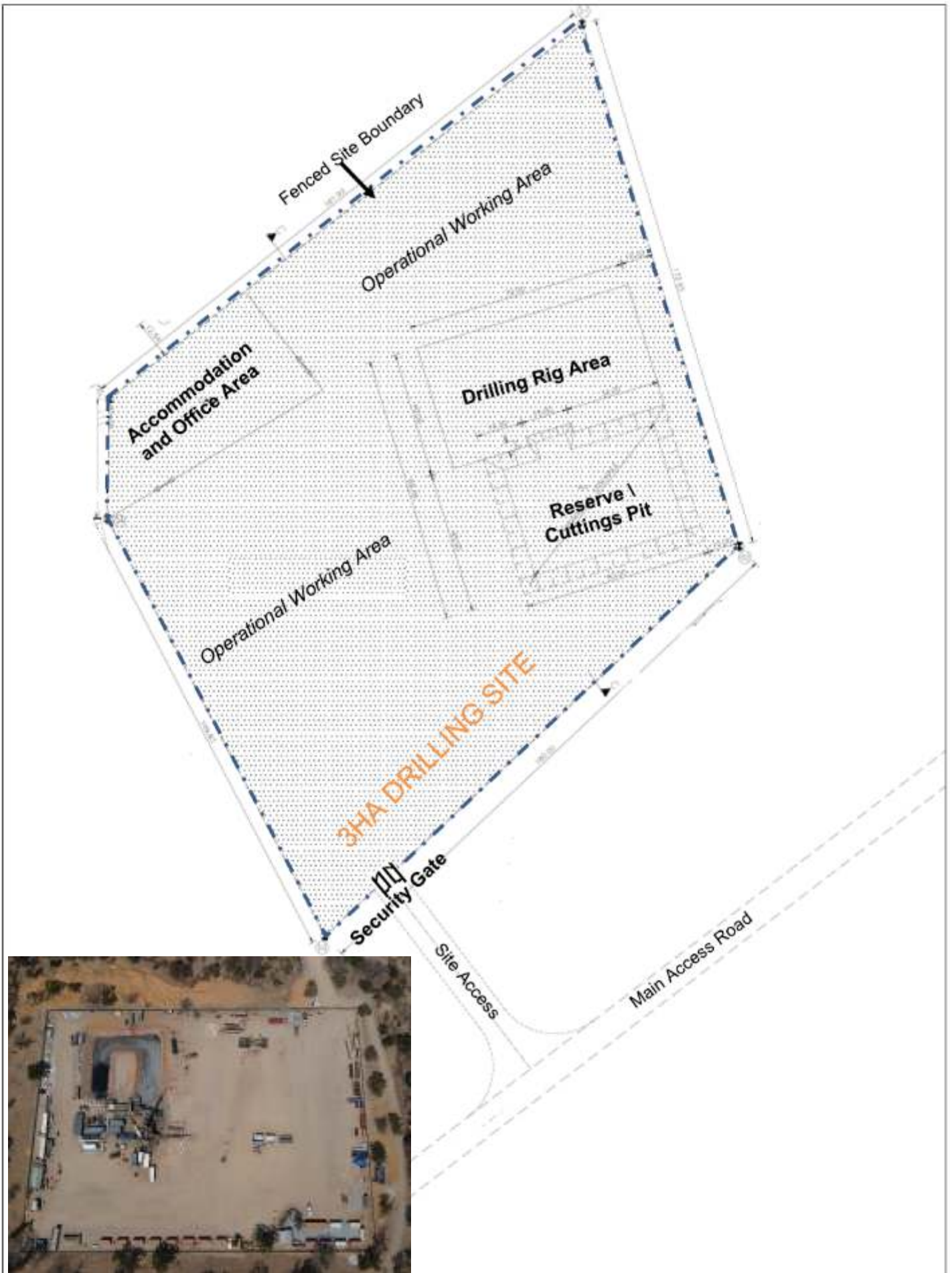
Figure 3.3: Example of a typical 3Ha footprint site coverage showing a general drilling site layout adopted for the drilling of multiple exploration and appraisal wells within the AOI in PEL No. 73.
