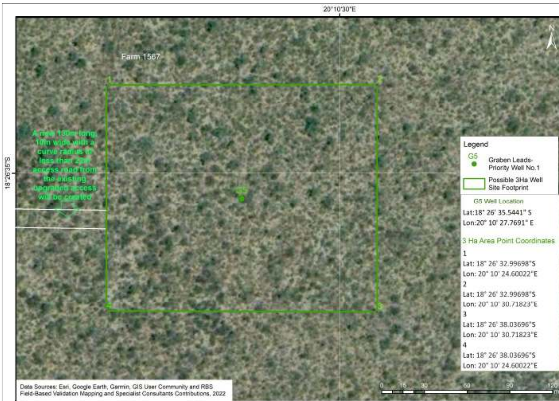
Figure 1.25: Detailed outline of the 3Ha area of the priority 1 covering the Karoo Rift Fill and Intra-Rift Fault Blocks Leads proposed exploration and appraisal well location No. G5 located on commercial farms on communal land, Farm No. 1567. A new 130m long, 10m wide with a curve radius of less than 22m access road from the existing upgraded access road will need to be created.
