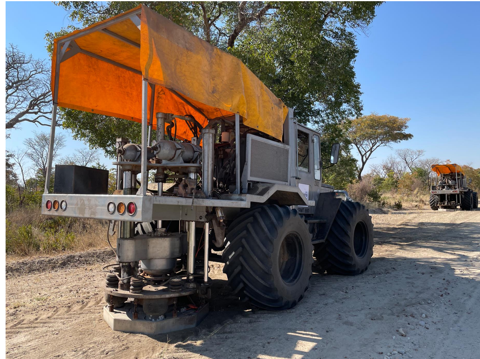
Polaris 860 Seismic Tractor : One of lightest impact seismic source equipment available
