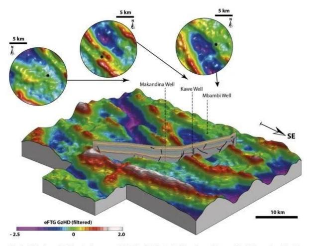
Fig.1: This is a <u>3D block diagram of GzHD</u> (High Definition Gravity), residual filtered grid of the gravity data. The hot colours (white and red) show structural highs, cool colours (blue and purple) show structural lows. Note the insets showing the three stratigraphic wells drilled to date, and the strong correlation of the 2D seismic line to the eFTG data.
