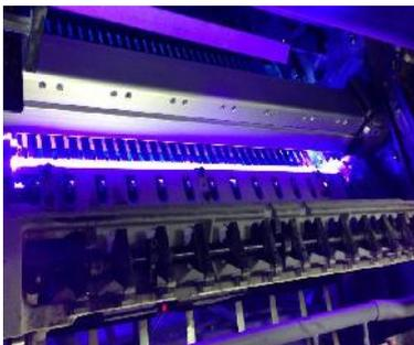
**UV curing** is a process in which ultraviolet light and visible light is used to initiate a photochemical reaction that generates a cross-linked network of polymers. UV Curing is adaptable to printing, coating, decorating, stereo lithography and assembling of a variety of products and materials owing to some of its key attributes, it is: a low temperature process, a high speed process, and a solvent less process. Cure is by polymerization rather than by evaporation.
