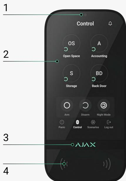
1. Ambient light sensor for automatically adjusting the backlight brightness.
