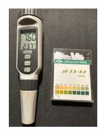
If the water's pH drops below 6.8, the enzymatic process slows and may stop. When this occurs, the reclaim water may turn light-brown and residual black sludge will become suspended processed water. Stopping the further transformation of complex organics into simpler substances.
