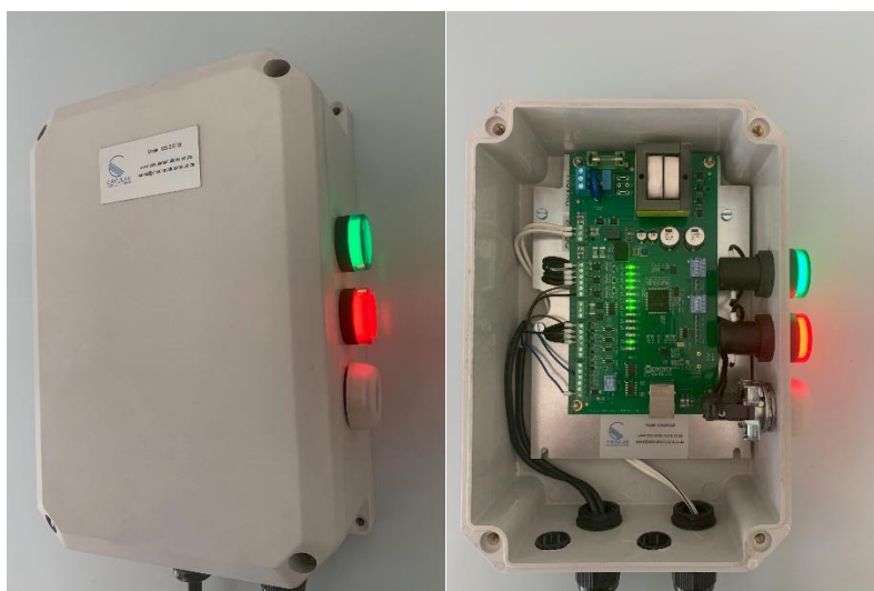
Figure 2.2 – Main Control Enclosures (closed and open)
