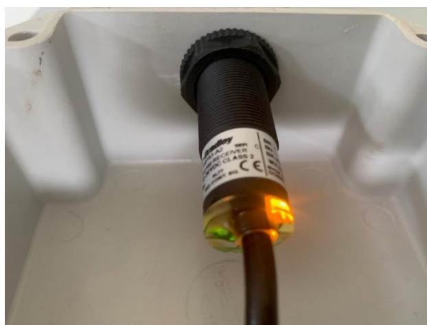
Figure 2.4 – Receiver sensor showing sensors are aligned
