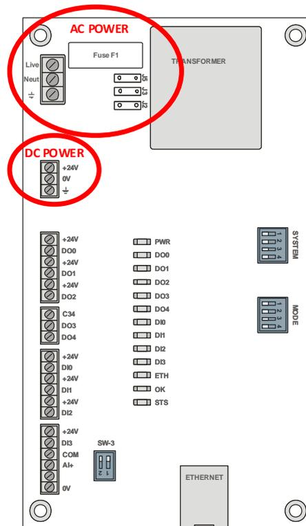
Figure 2.3 – AC & DC Power Circuits
