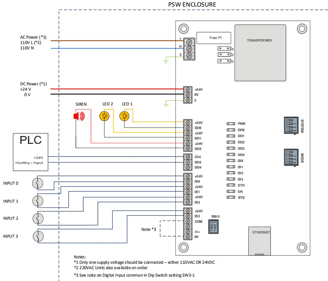
Figure 2.2 – Typical Wiring Diagram
