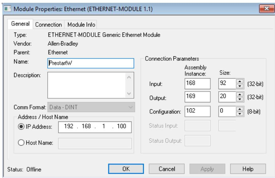
Figure 3.11 - RSLogix 5000 General module properties for Pre-start Warning
