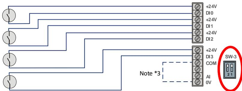
Figure 2.8 – Digital Input Wiring Example
