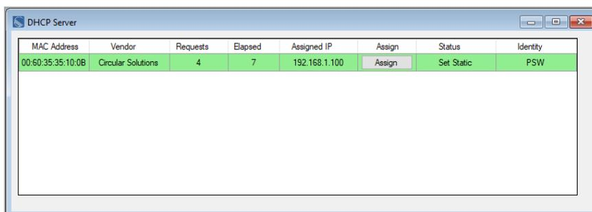
Figure 3.5. - Successful IP address assignment
