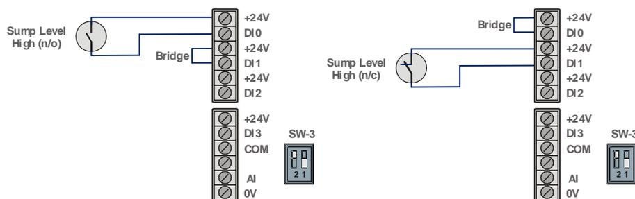
Figure 2.11 – Example of wiring to trigger device for n/o or n/c contact
