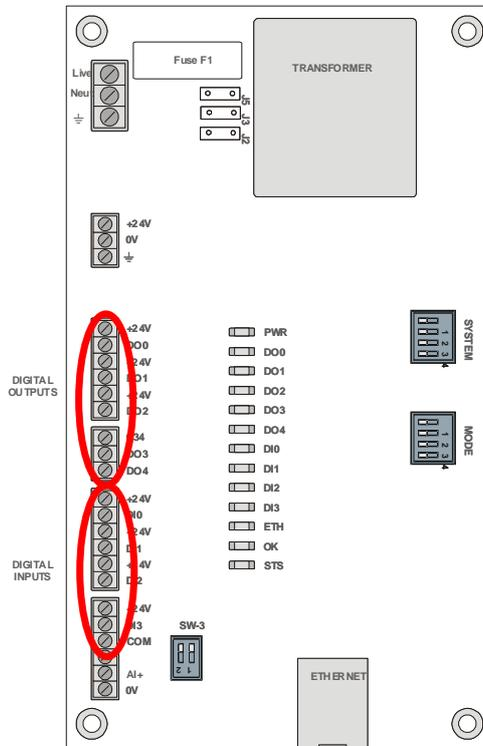
Figure 2.7 – Input and Output Connection
