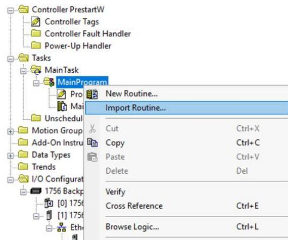
Figure 3.14. – RSLogix 5000 Importing Pre-start Warning specific routine and UDTs
