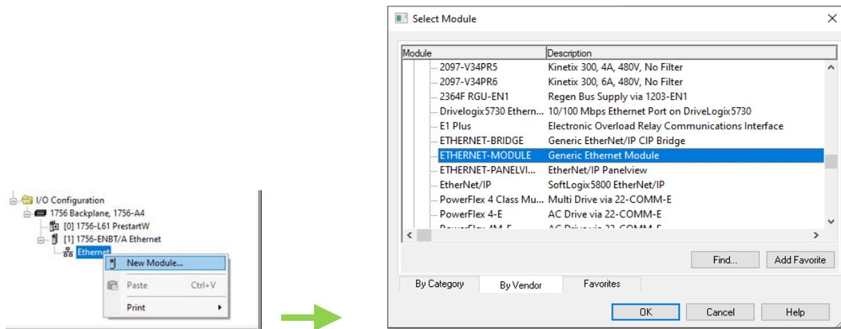
Figure 3.10 - Add a Generic Ethernet Module in RSLogix 5000
