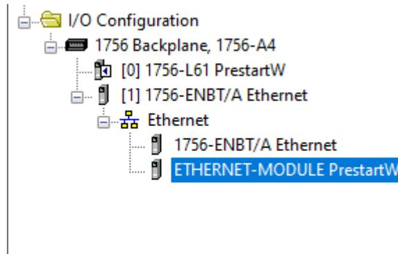
Figure 3.13 – RSLogix 5000 I/O module tree
