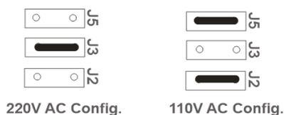
Figure 2.6 – AC Power - Jumper Configuration
