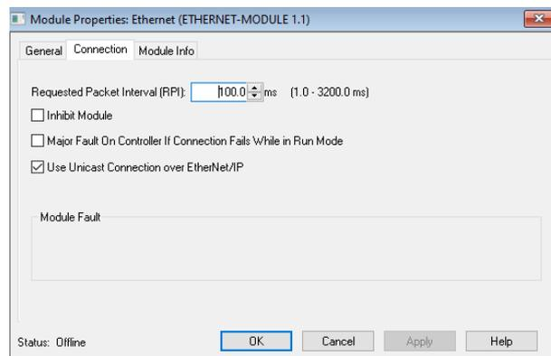
Figure 3.12 - Connection module properties in RSLogix 5000
