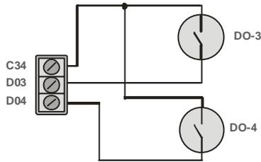
Figure 2.9 – Common Internal Connections of DO3 and DO4
