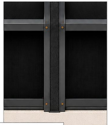
DETAIL B – RECOMMENDED SCREEN CLOSURE
