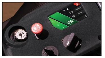
DIGITAL CONSOLE FOR DIAGNOSTICS Get into action quickly if something breaks. The console tells you the error
