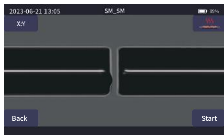
Uneven end face of optical fiber
