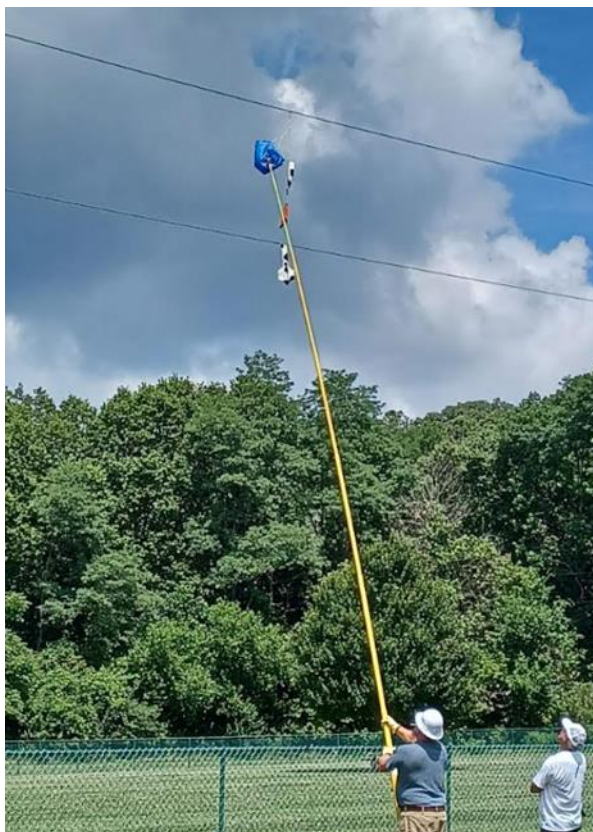
Attempting a ground retrieval with a 100kilavolt rated lineman stick
