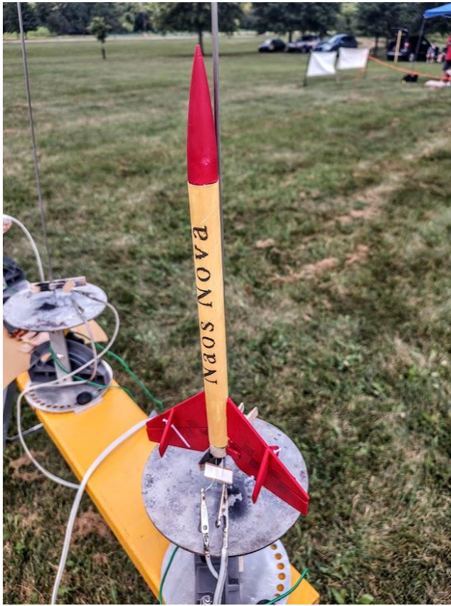
Fins that fold out after apogee
