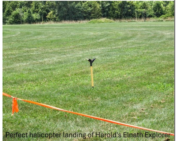
Yes, it is supposed to do that! Helicopter fins give a soft nosecone-first landing
