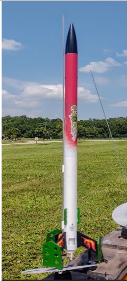
Jeremy's Slo-Mo with purposely cocked fins designed to cause it to spin in flight.
