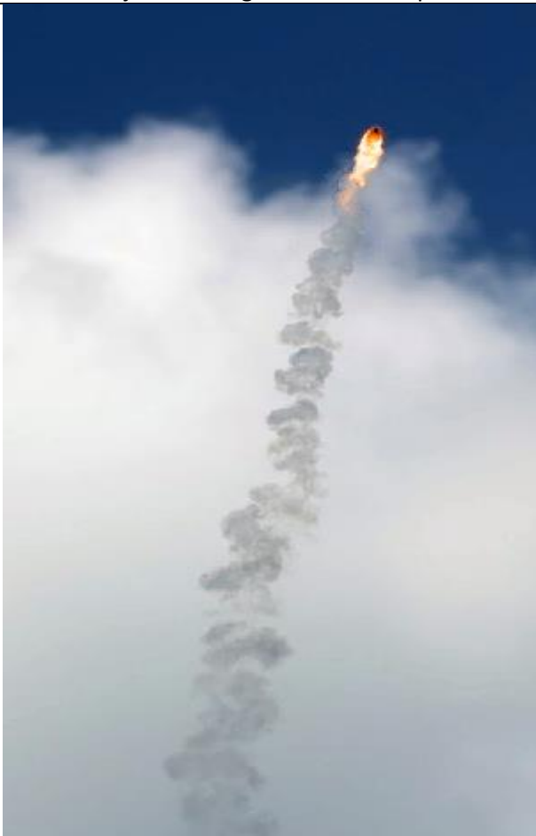
V2 CATO (Catastrophy On Take Off) due to a bad motor
