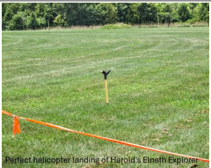
Yes, it is supposed to do that! Helicopter fins give a soft nosecone-first landing
