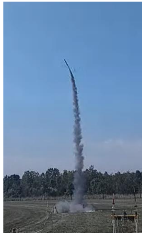
F23-4FJ bad motor, fours old, smoke is good, arc is bad....
