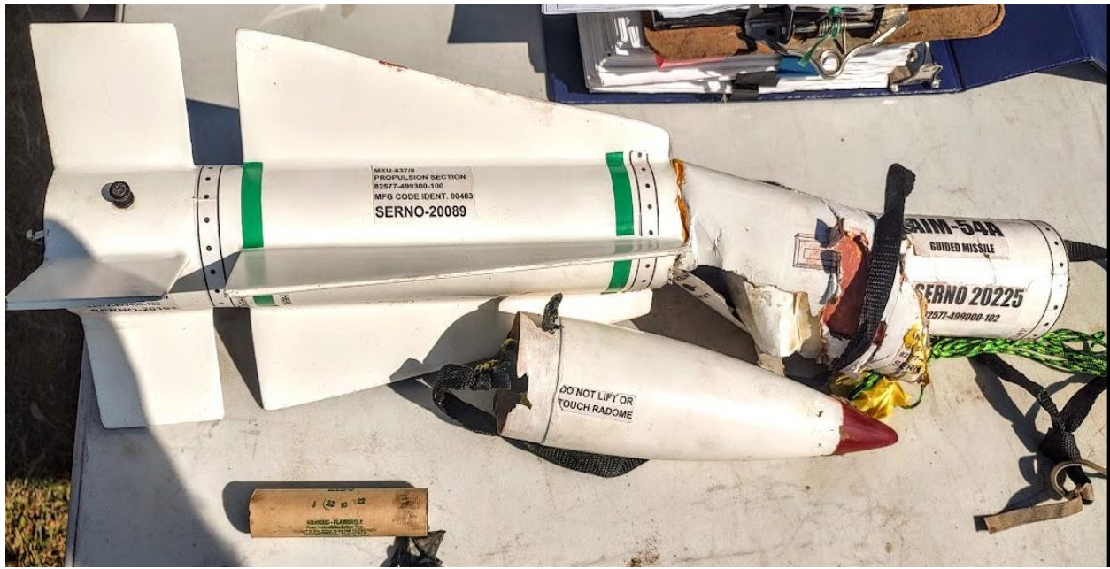
Rick's AIM-54A . A bad E12-6 motor caused the failure.
