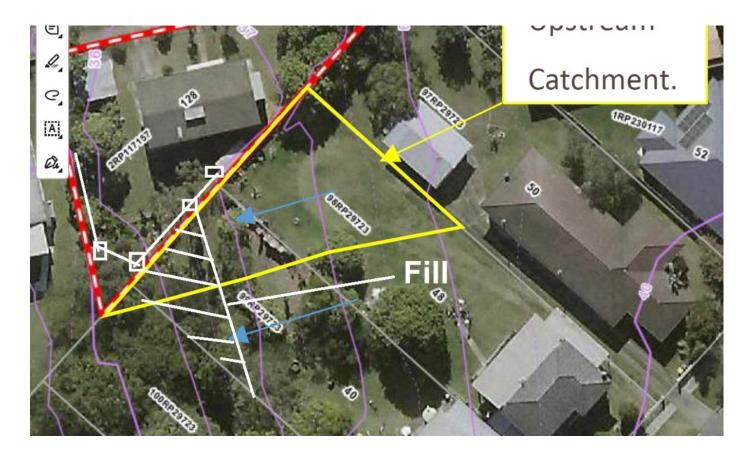
Above – sketch prepared by Manteit demonstrating that fill required by owner for Civil Works concept plan to work to obtain lawful point of discharge to command the lot.
