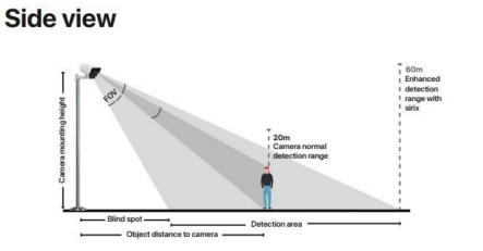
This graphic shows the extended detection range of the camera when set to its broadest angle (2.8 mm or 90° HFOV).
