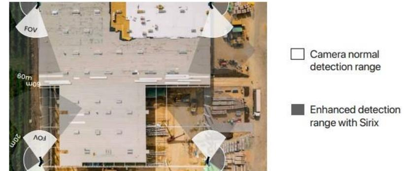
This top-down graphic shows the expanded detection area of the camera with Sirix enhancement, when set to its widest angle (**2.8 mm or 90° HFOV**).
