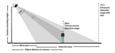
This graphic shows the extended detection range of the camera when set to its broadest angle (2.8 mm or 90° HFOV).
