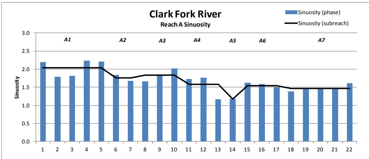
Figure 2-8. Reach A sinuosity for Phases (bars) and Subreaches (line).
