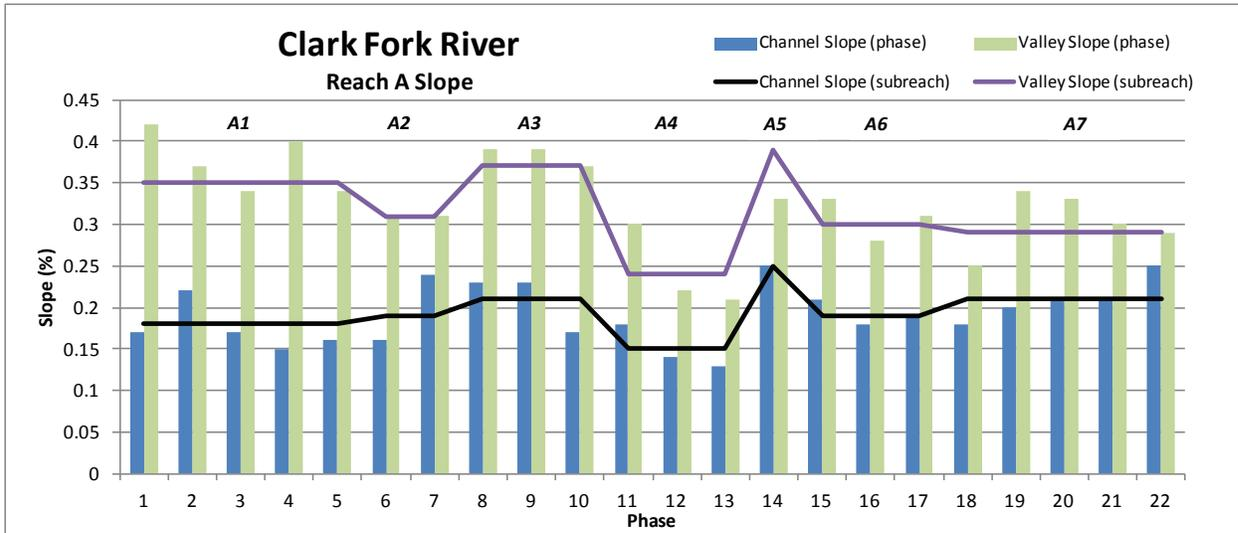
Figure 2-7. Channel and valley river slope for Reach A Phases (bars) and Subreaches (lines).
