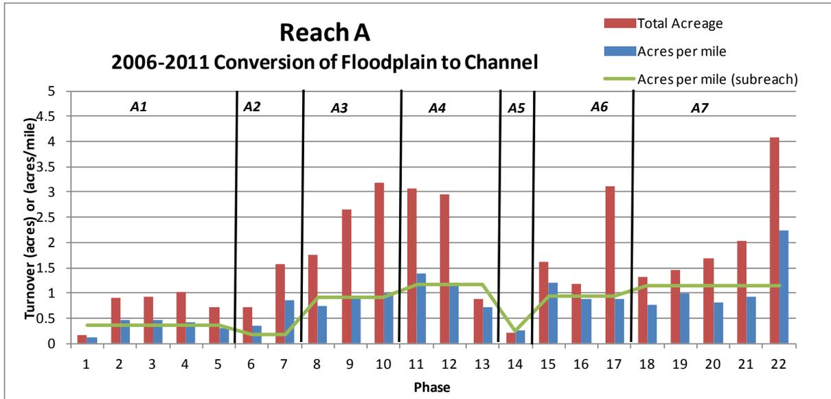
Figure 2-13. Bank erosion acreage (conversion of floodplain to channel), 2006-2011.
