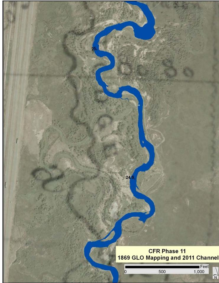
Figure 2-3. Example of deviation between 1869 GLO map and modern channel (blue), including a section line crossing, Phase 11.
