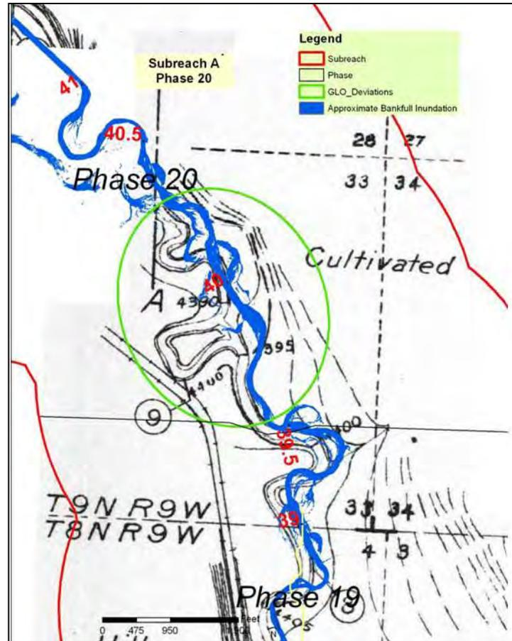
Figure 2-6. Example of deviation between 1914 channel (Marshall, 1914) and modern channel, Phase 20.
