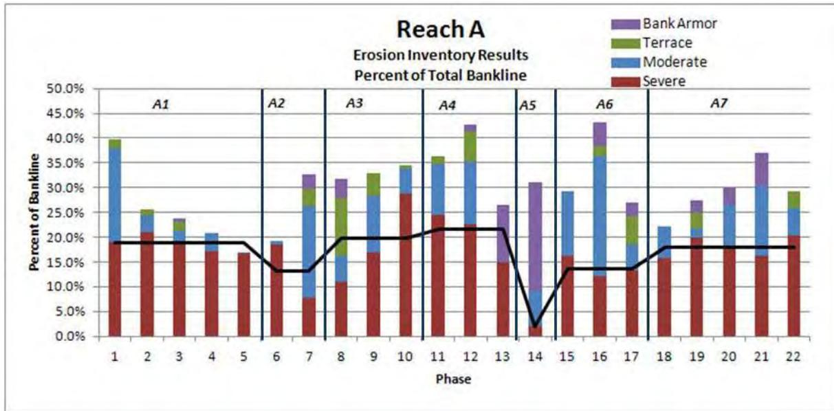
Figure 2-9. Rapid erosion inventory results, Reach A; black line is severe erosion by Subreach.
