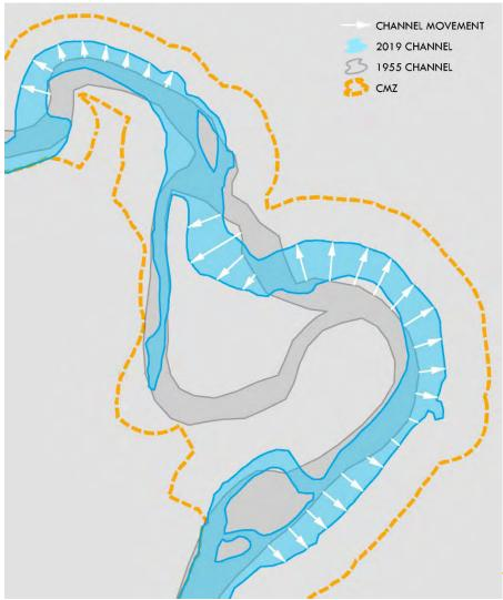
With a few refinements, this CMZ defines a base remedy area where all contaminated sediments will be removed.
