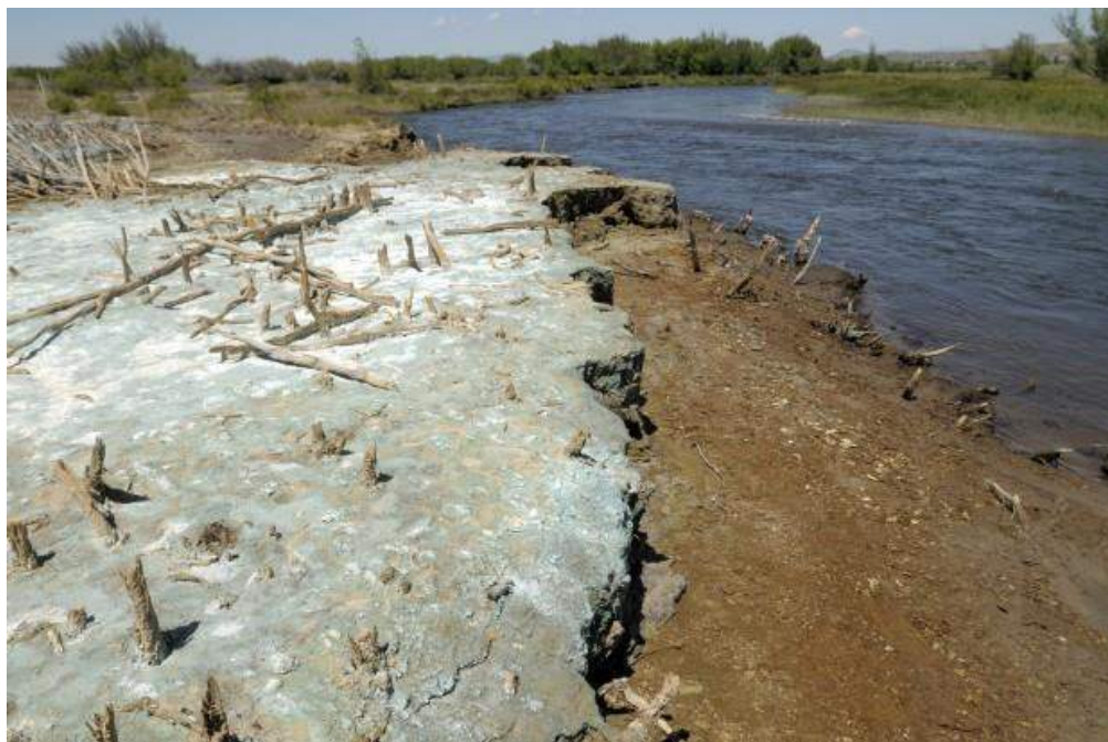
Figure 23- A “slicken” of toxic waste deposited on the riverbank of the Upper Clark Fork River near Racetrack. Photo source: Tom Bauer of the Missoulian . These dense, toxic mats of contaminated soil have inhibited plant growth for more than 100 years and continue to leach heavy metals into the river.
