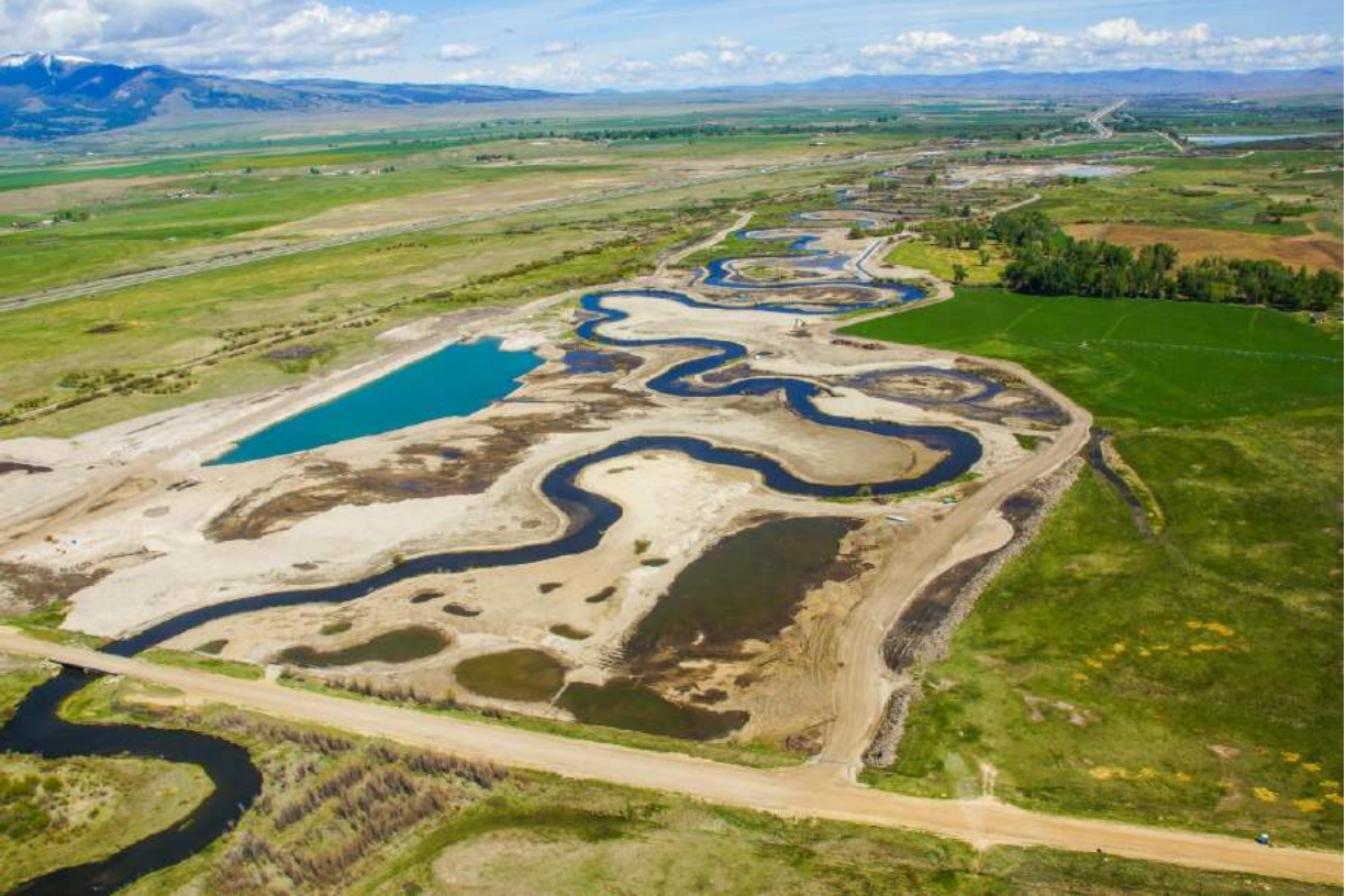
Figure 36- Aerial photo of the remediation and restoration of Phases 5 and 6 (part of the Upper Clark Fork River Reach A). This photo is facing due south from Galen Road (at the bottom of the picture) near the Dry Cottonwood Creek Ranch which is operated and owned (part owners) by the Clark Fork Coalition. White patches indicate where contaminated soil has been removed and hauled away. No remediation was carried out in the river (just banks and floodplain), and its natural course was left intact. The light blue “pond” is where source gravels were removed to help rebuild parts of the floodplain. Smaller potholes in the foreground were added as wetland features to help improve habitat diversity in the recovering floodplain. In 2016 hundreds of migrating snow geese were observed using these features.
