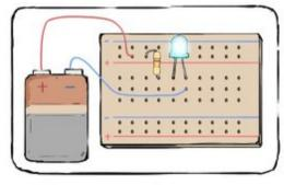
Connect the wire next to the resistor to the positive side of the battery.
