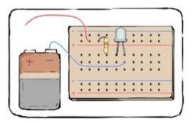
Connect the wire next to the short leg of the LED to the negative side of the battery. Step 5
