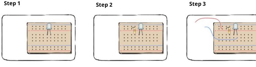
Fix the LED to the breadboard.
