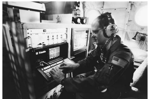
A crew member aboard an aircraft belonging to the Hurricane Hunters prepares for a dropsonde launch. As they fall through a tropical cyclone's rain bands, dropsondes collect detailed information about the system, thereby providing more data for forecasting and emergency management purposes. (NOAA)
